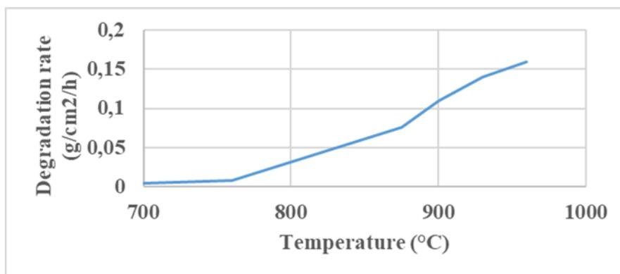
**Figure 11. Degradation rate as a function of contamination temperature.**
